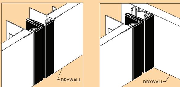
1. Install the architectural joint system on a level wall surface. This may require adding leveling compound to raise the tops of the frames.
